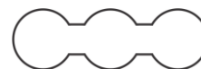
Image 2. Most adequate \mu PAD layout found for simultaneous analysis with linear geometry 8.25 mm diameter circular reactional zones and 2.0 x 4.12 mm hydrophilic channels
