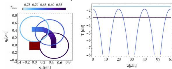
**Image 3.** Device transmittance for final positions – taper touching the waveguide. Curve for taper center final positions with the transmittance for  $z=0$  represented by the color scheme (left). Transmittance as a function of interaction length for the three respective situations depicted on left (right).
