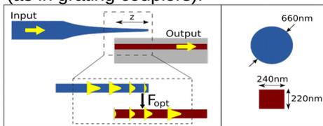
**Image 1.** Schematic of the coupler concept. Blue represents silica, red, silicon and yellow, power and modal profile. Light is launched in a 660nm diameter tapered fiber and coupled to an integrated waveguide with 240nm width and 220nm height. The fiber is subject to an optical force that aligns the system.
