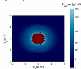
**Image 2.** Acceleration in g's ( $g=9.8\text{m/s}^2$ ) for a silica cylindrical rod under the optical force for 1mW of input power. In red is represented positions not allowed for the fiber taper center due to the waveguide's presence at the origin. For a distance of  $1.25\mu\text{m}$  the optical force corresponds to 1g and is rapidly increasing as  $q$  decreases.
