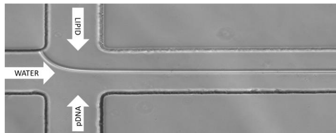
Figure 1 – Microfluidic device used to perform the complexations
