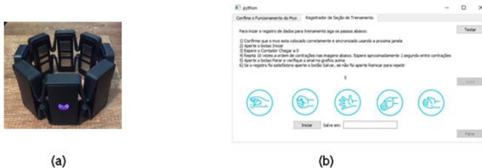
Figure 2. (a) The Myo Armband. (b) Screen capture of the program used to perform the data acquisition of EMG signals to perform the first classification experiment.
