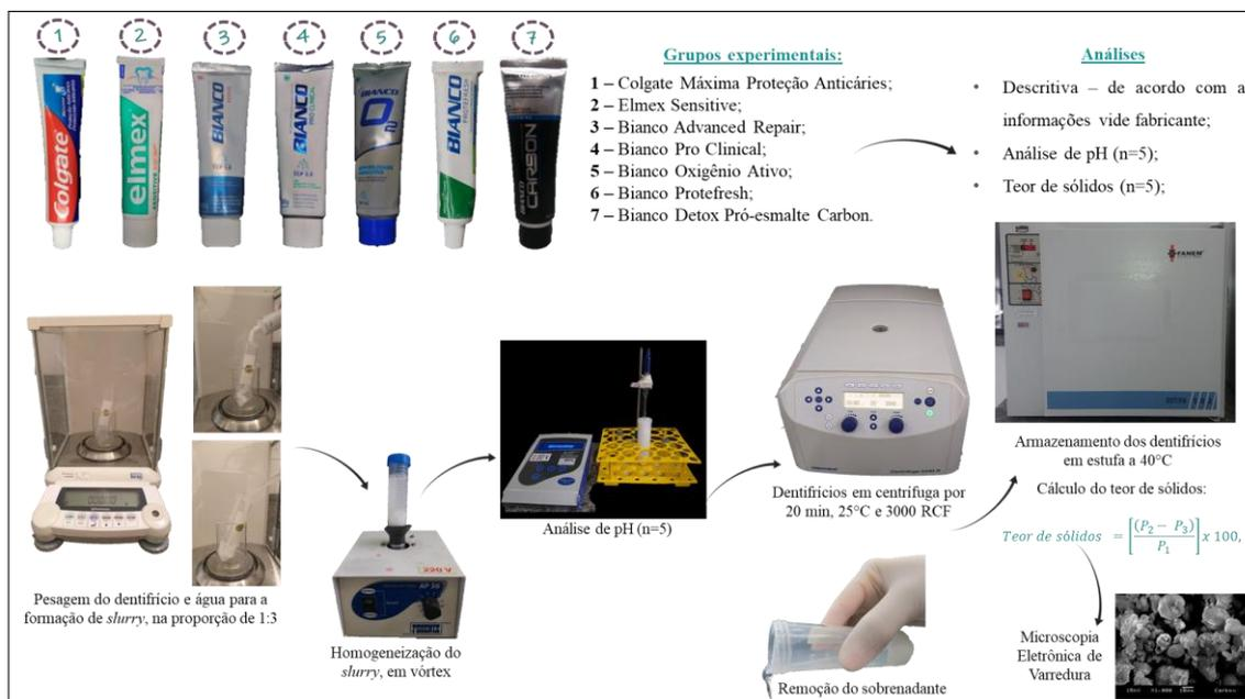
**Figura 1.** Fluxograma experimental.
