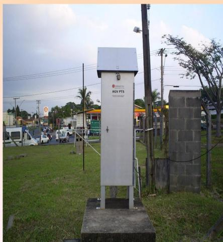
Fig. 1: Amostrador de Grande Volume (AGV-PTS)
