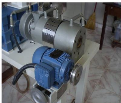
Figura 1: Extrusora INBRA LABOR PQ-30
