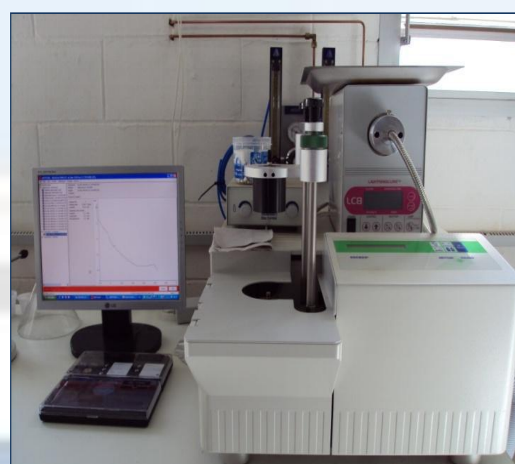
Figura 2: DSC – Differential Scanning Calorimeter, modelo DSC-823e, marca Mettler Toledo.
